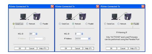
Choose the interface—serial, network, or parallel cable communications—you want to use for connecting to this printer:
